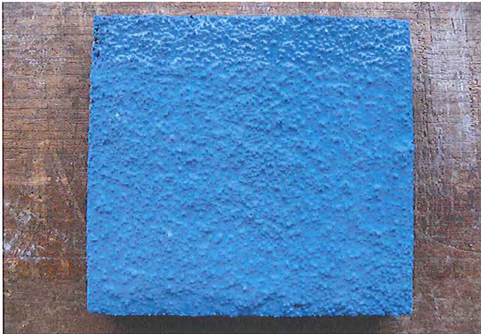
Figure 2. Image of specimen 243982/47 after artificial weathering
